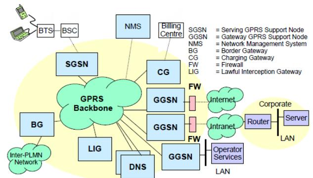
Fig. 3 Architecture of GPRS connection [9]
