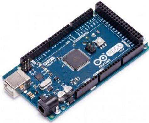
Fig. 4 Arduino Mega 2560 (Fig 4) microcontroller
