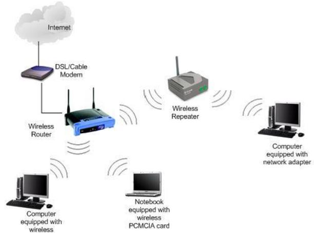
Fig. 2 Architecture of Wi-Fi network connection
