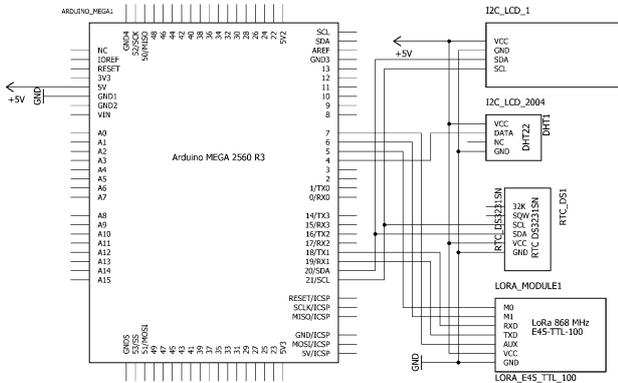
Figure 2. Schematics of development board and communication module
