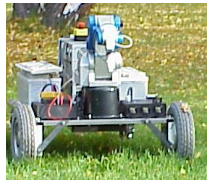
Fig. 2. Prototype of the mobile platform with articulated robot without ultrasonic measurement lay out
