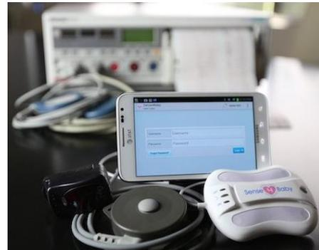
Figure 2. Sense4Baby Prenatal Monitoring System
