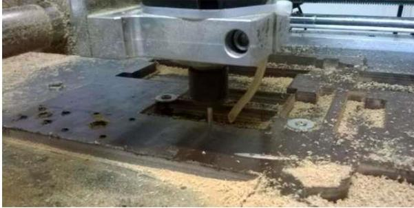
Fig. 5. Construction of Bakelite carriers using a CNC machine
