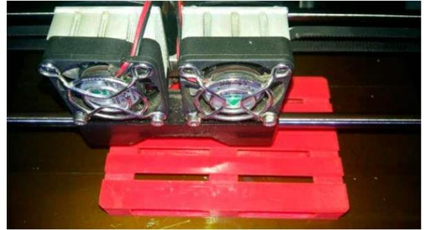
Fig. 7. 3D printing of pallets
