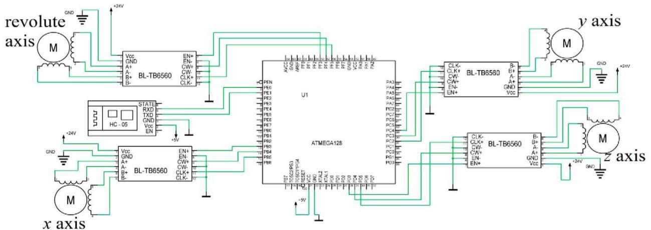
Fig. 8. Electrical schematic of the automated warehouse
