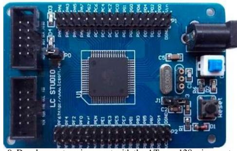
Fig. 9. Development environment with the ATmega128 microcontroller
