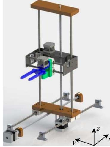
Fig. 3. Virtual model of the Cartesian manipulator
