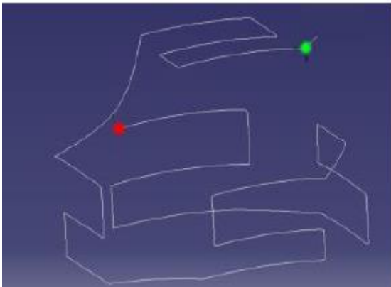
Fig. 9. The electric motor painting: trajectory for control box.
