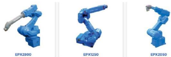
Fig. 4. Robots applicable for painting [5].
