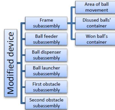
Fig. 3. Mechanic structure of the modified device
