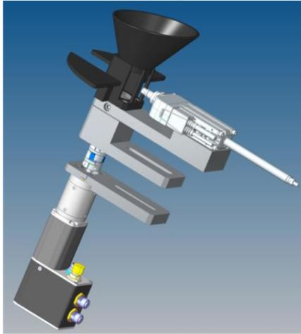
Fig. 9. Ball launcher subassembly
