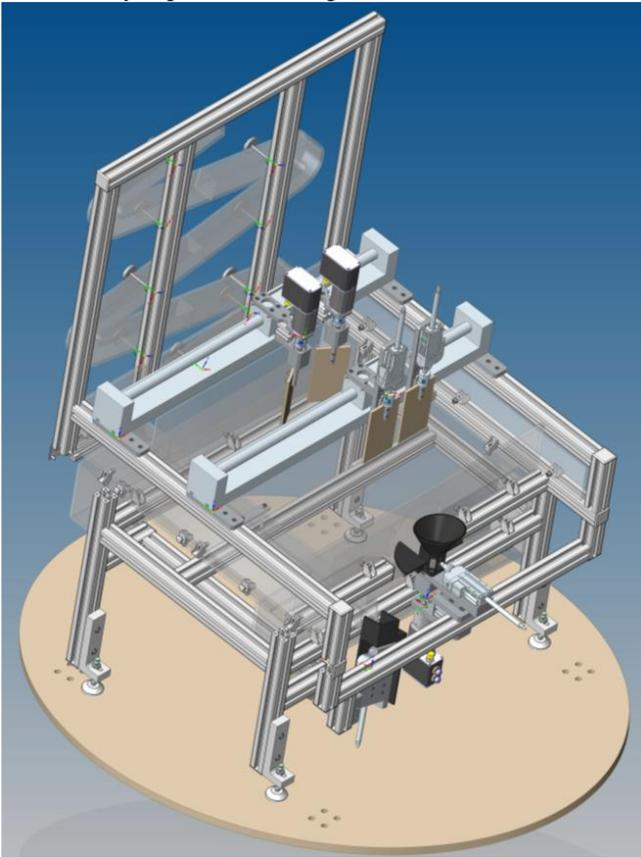
Fig. 4. Mechanic structure of the modified device
