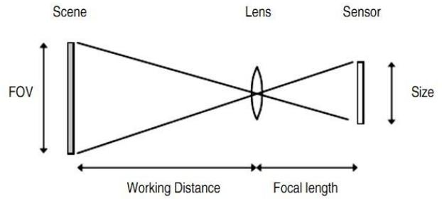
Fig. 2. Determining focal length and sensor size [2]
