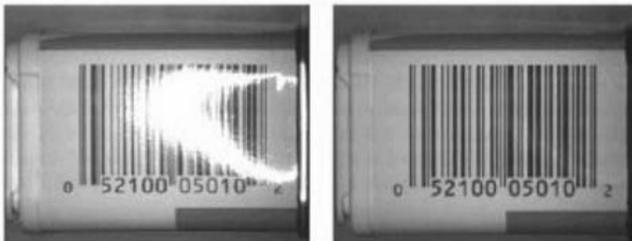
On the left part of the image the barcode image was acquired using highly directional light and the barcode on the right side was acquired using diffused lighting to reduce glare. [2]
