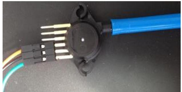
Fig. 8. Pressure sensor MPX4250AP
