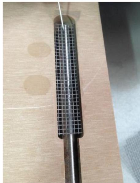
Fig. 3. Preparation of the silicone rubber finger, adding the mesh
