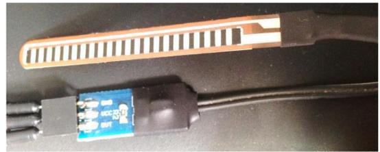
Fig. 7. Flex sensor used for the test soft robotic finger
