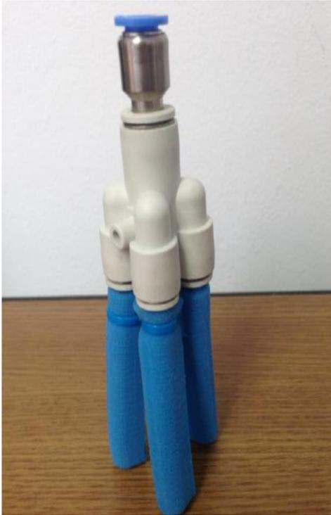
Fig. 1. Proposed silicone based soft robotic gripper
