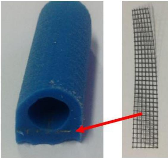
Fig. 5. Cross-section of the silicone rubber soft finger, it can be noticed the reinforcement mesh
