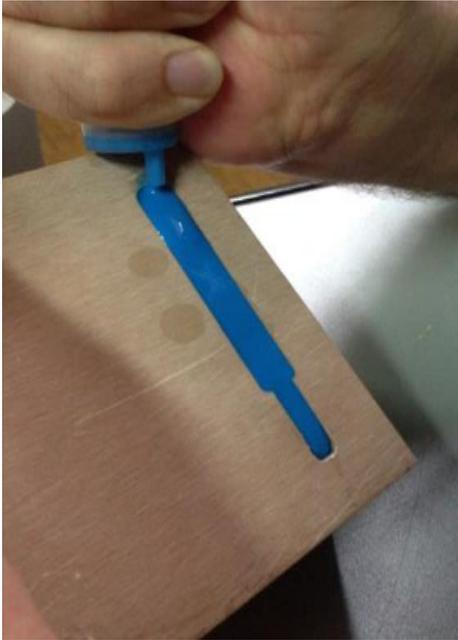
Fig. 4. Obtained silicone based soft finger
