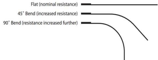
Fig. 6. How it works principle for flex sensor [22]
