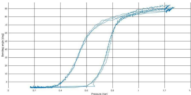
Fig. 9. Correlation between pressure and bending for 3 cycles of the soft robotics finger
