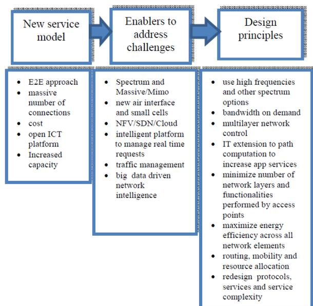
Fig. 3 New communication model.
