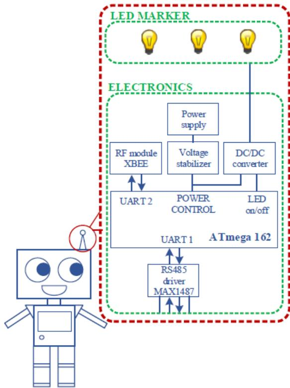
Fig. 6 Structure of the active LED beacon.
