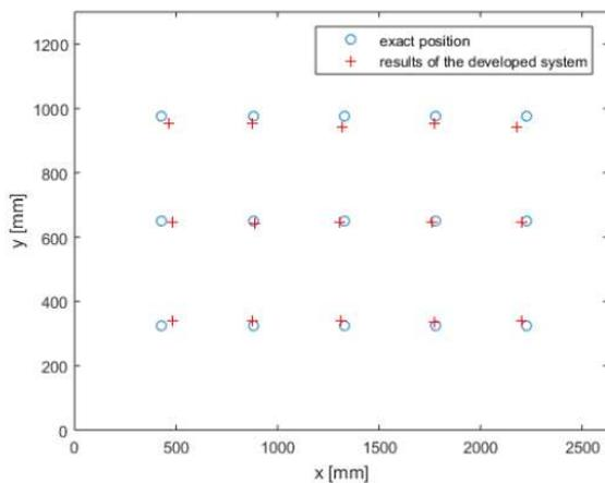
Fig. 8 Results of static testing: blue circles denote actual positions measured by the referent localization system and red crosses represent the output of the developed system.
