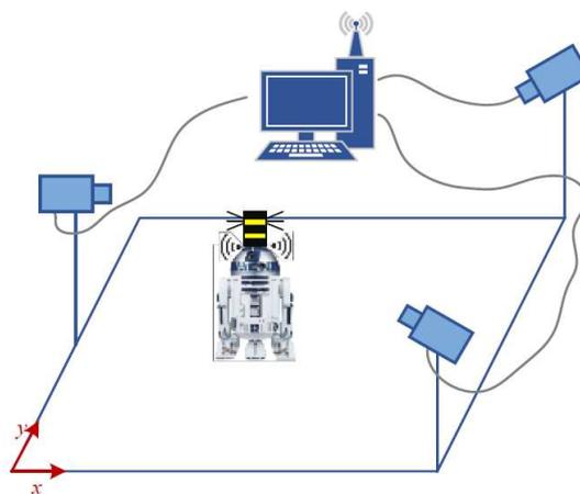
Fig. 1 Design of the localization system.
