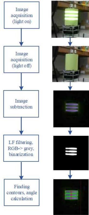
Fig. 3 Image processing algorithm.
