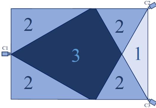
Fig. 2 Playground coverage. The lightest part is covered by one, darker by two, darkest by three cameras.
