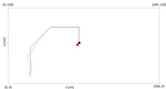
Fig. 9 Results of the testing: black line denotes actual position measured by the referent localization system and red line represents the output of the developed system.
