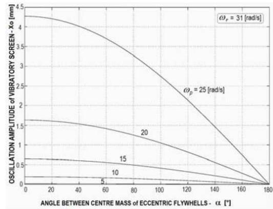
Fig. 9 sub-resonant characteristics of vibratory screen ( $\omega_p < \omega_r$ )
