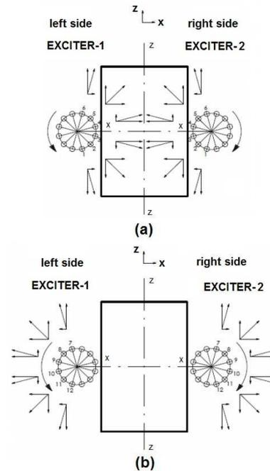
Fig. 4 The vector diagrams of excitation forces; (a) force to axis, (b) force from axis
