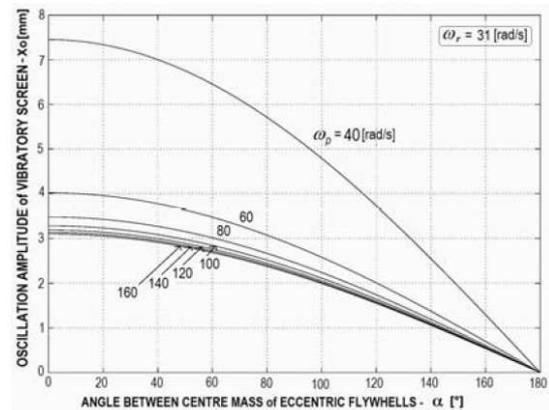
Fig. 10 The super-resonant characteristics of vibratory screen ( $\omega_p > \omega_r$ )
