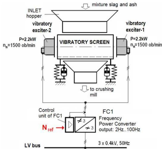
Fig. 5 The block scheme of open-loop control (sensor-less) of unbalanced vibratory exciters (unbalanced motors)
