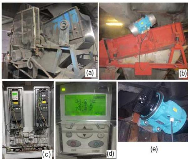
Fig. 11 The real image show of realized regulated drive of one vibratory screen; (a) old system (unregulated drive), (b) new system with unbalanced vibratory excites, (c) frequency power converters FC1, FC2, (d) operator control panel (e) unbalanced motor with eccentric unbalanced flywheel.
