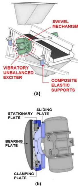
Fig. 2 The final solution of vibratory screen with unbalanced motors; (a) layout of entire system, (b) swivel mechanism in unbalanced exciter
