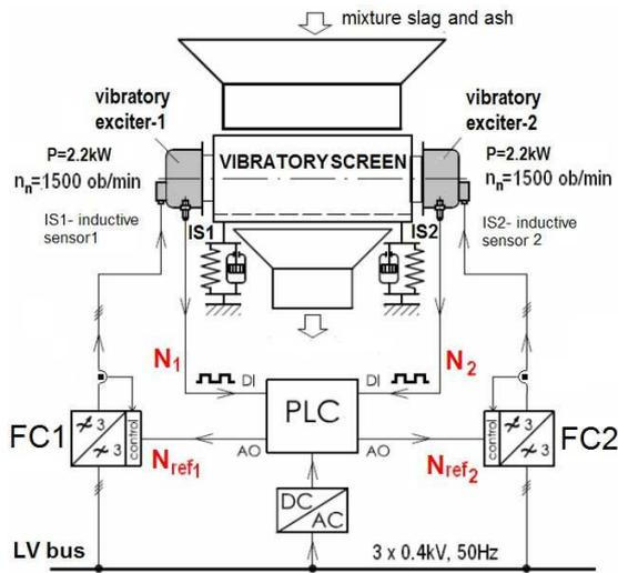
Fig. 6 The block scheme of close -loop control of unbalanced vibratory exciters (unbalanced motors)
