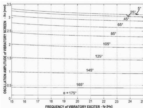
Fig. 8 The family of amplitude-frequency (AF) characteristics of regulated drive of vibratory screens in the super-resonant range (operating characteristics)
