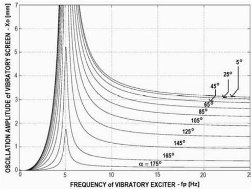
Fig. 7 The family of amplitude-frequency (AF) characteristics of regulated drive of vibratory screens
