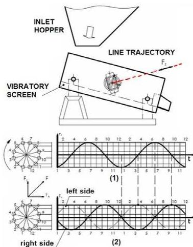
Fig. 3 The principle of realisation of linear oscillation of vibratory screen
