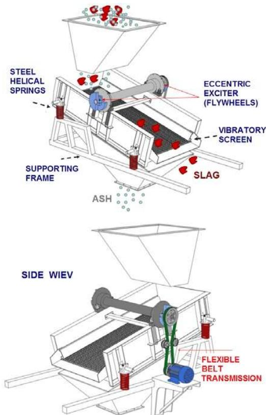
Fig. 1 The drive of old system of vibratory screens on thermal power plant TENT-B
