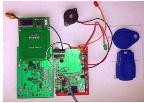
Fig. 2 RFID elements in the system for the recording of work hours and the control of access
