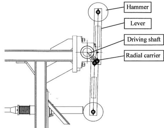
Fig. 1 A Basic construction elements of the mechanical rapping device important for the analysis
