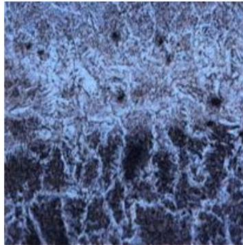
**Location:** Heat affected zone of welds - vertical carrier (HAZ)
